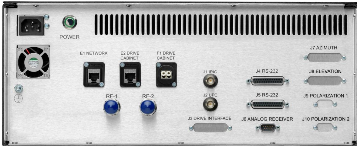
Figure 1-2 Power switch and data connections — specifics vary by system, see Appendix 2: ACU Rear Panel Connections.
