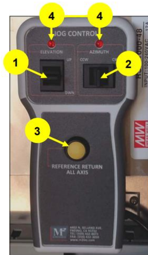
Figure 4-2 Jog controller provided with the M 2 ACU-X2PFM-C230. (Not the same as the handheld PMCU made by Radeus Labs.)
