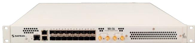
**The WR-Z16 is the reliable precise time fan-out for White Rabbit distribution on 1G Ethernet-based networks. It is a standalone device with 16 SFP connectors which provides sub-nanosecond accuracy time over plug-and-play fiber links.**
