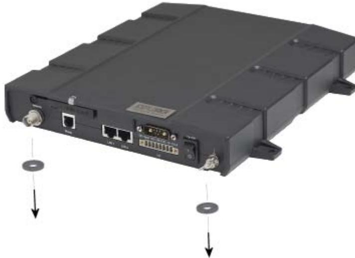
2. Fasten the Basic cable support to the terminal using two M4 x 6 mm countersunk screws.
