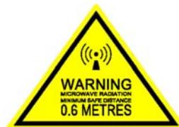
The minimum safety distance is 0.6 m to the side and above the antenna when the EXPLORER 325 is powered. The safety distance of 0.6 m does not apply directly below the antenna, as the radiation forms a hemisphere above the antenna.
