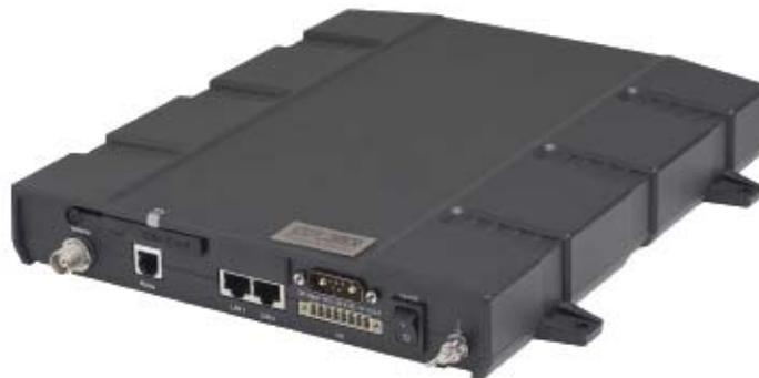
The terminal supplies 23.0 - 30.0 V DC to the antenna through a single coaxial cable. The DC input for the terminal is designed for both 24 V DC and 12 V DC power supply.
