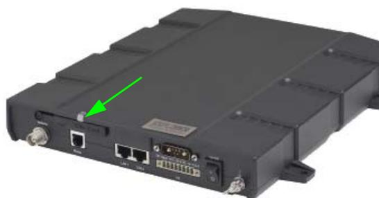
2. Insert the SIM card into the SIM slot. Place the card with the chip side facing up as shown.
