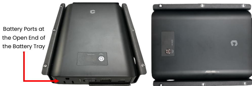
Figure 3: Place the ChargeTech battery pack into the battery tray. (Bloodhound G1)
