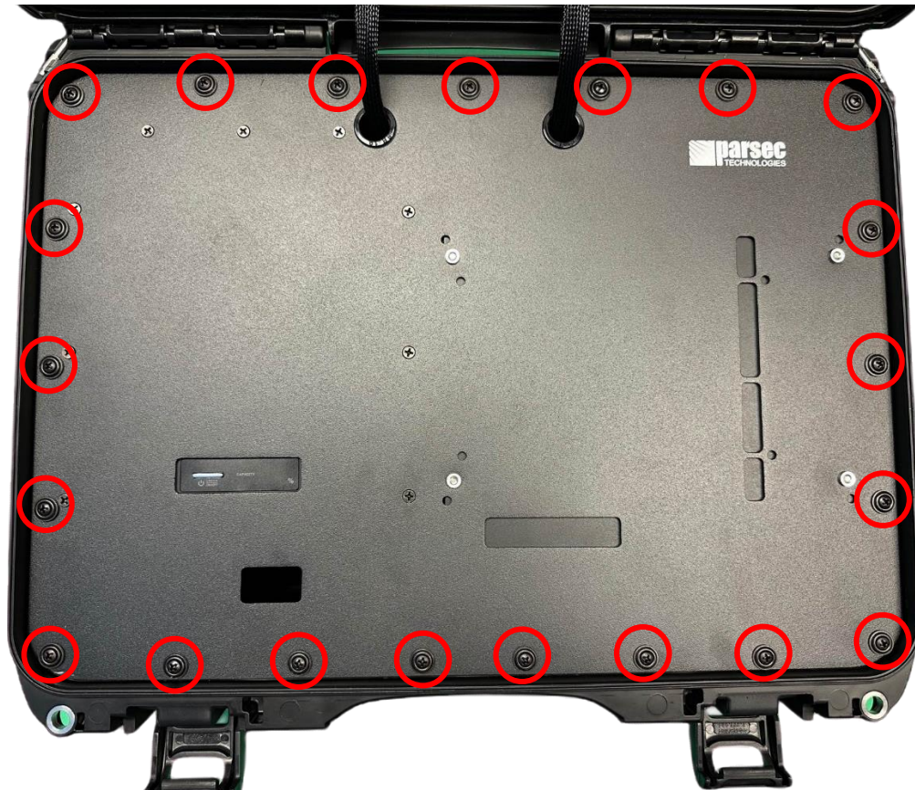
Figure 24: Fasten the cover plate to the case using PTA0351 screws.
