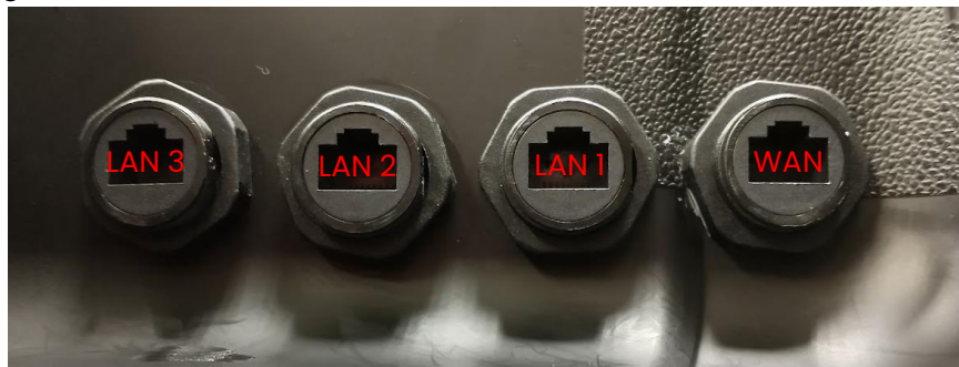
Figure 18: Connect the router to the RJ-45 ports on the case using ethernet cords.
