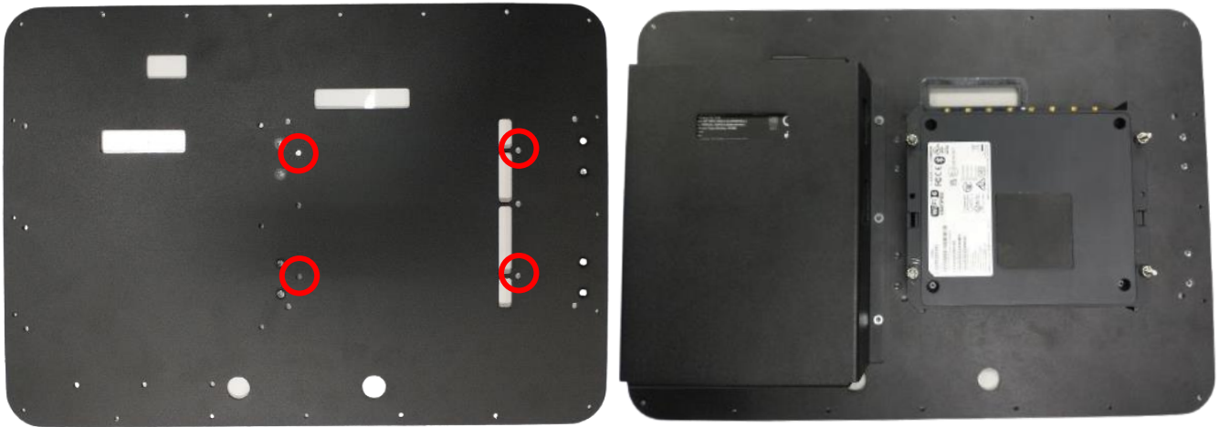
Figure 9: For R1900 router, fasten the router to the cover plate using PTA0579 screws, PTA0140 washers, PTA0844 lock washers, and PTA0408 nuts.
