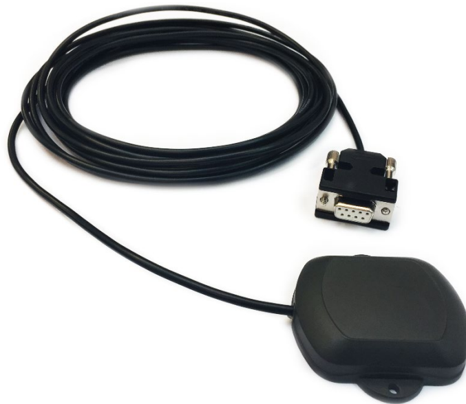
Figure F.1: GPS antenna
