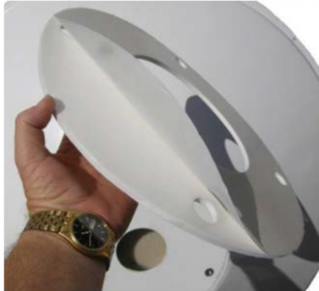
Figure 2.20: Sticky side of the mounting pad.
