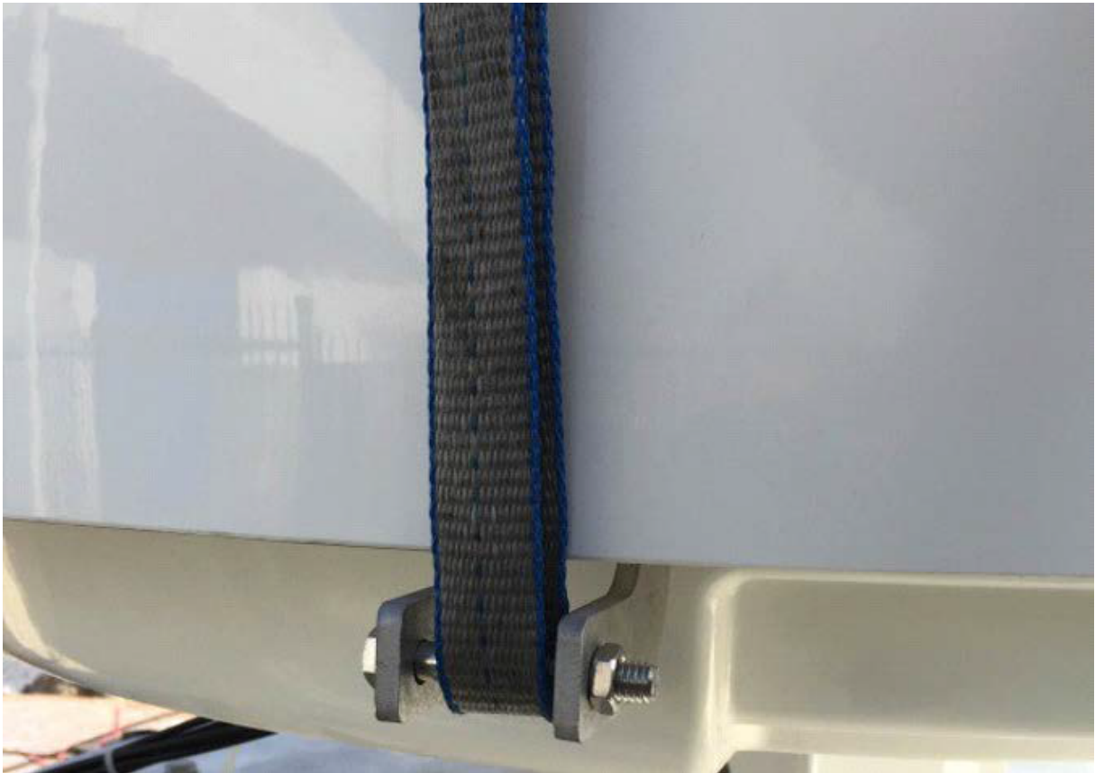
Figure 2.19: Horizontal bolt in lifting brackets.
