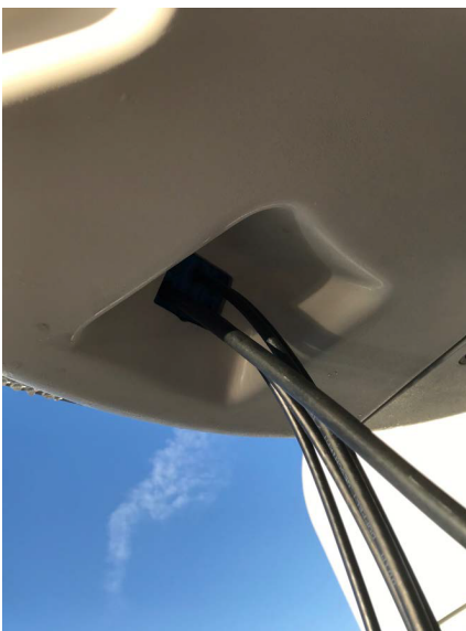
Figure 2.13: Blue cable seal module outside the radome bottom.
