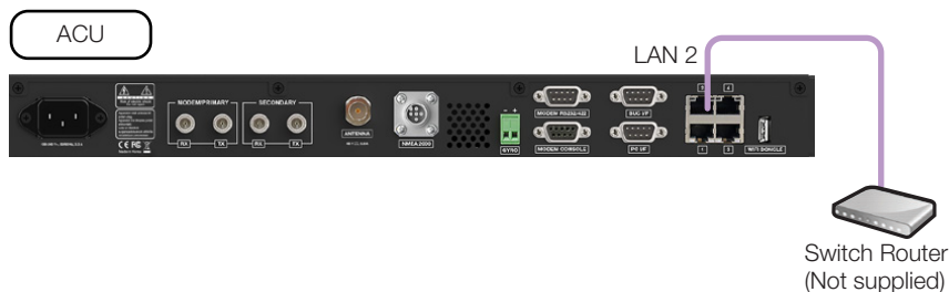
Figure 27: ACU to Switch Router Cable Connection
