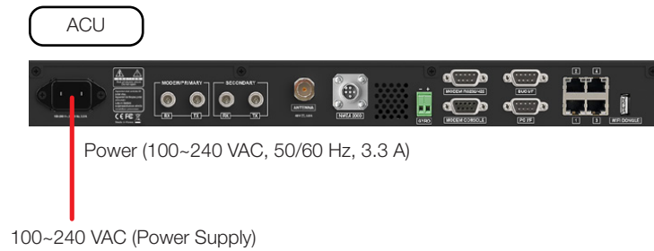
Figure 22: Connecting Power to ACU
