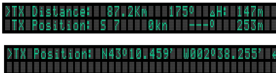
Figure 62: Transmitter GPS Information screen
