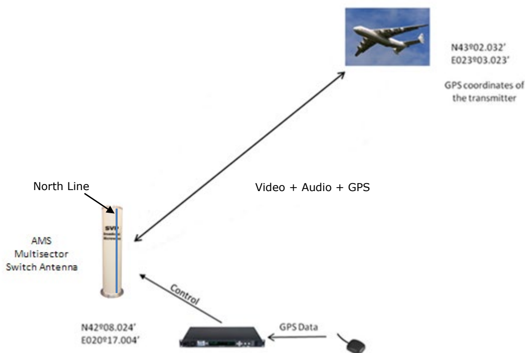
Figure 54: Autotracking with panel switching
