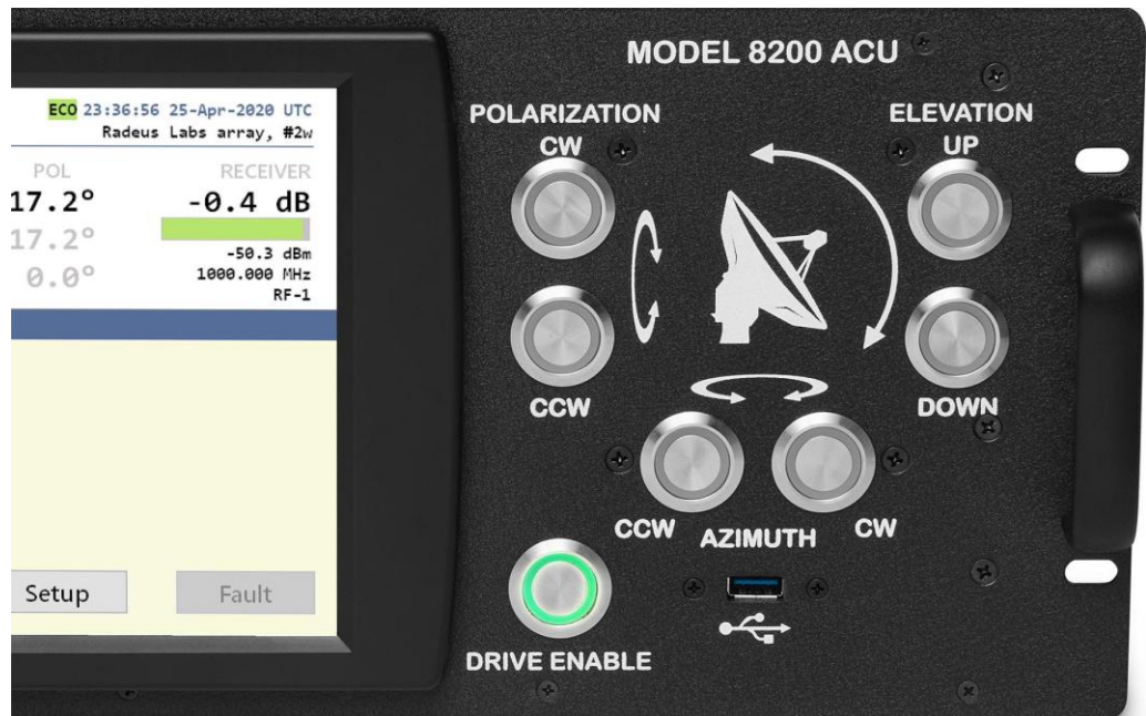
Figure 4-24 The ACU's hardware jog buttons have LEDs that show what the controller is doing. See Figure 4-24 and section 4.7.6, "Track Immediate, Manual Peaking, and Bias Angles" to adjust button behaviors.
