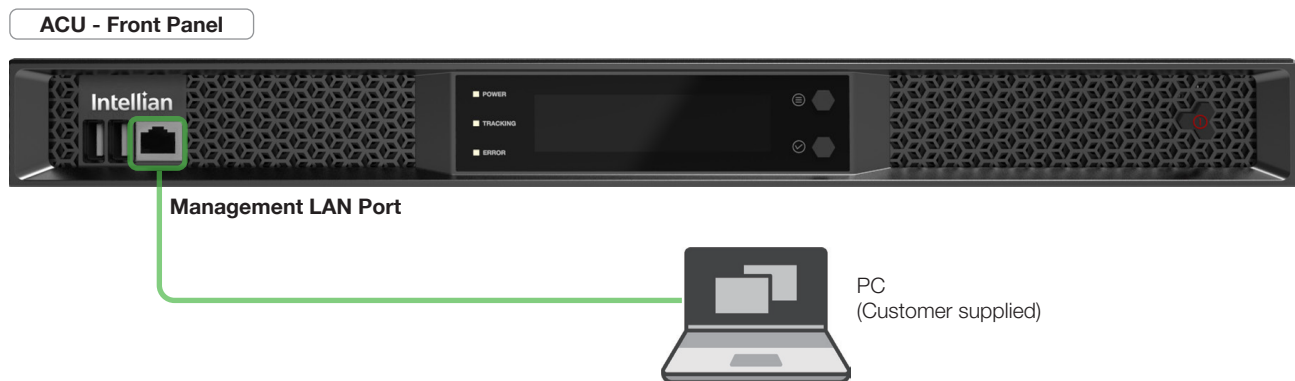
Figure 73: Front Panel Management LAN Port Connection
