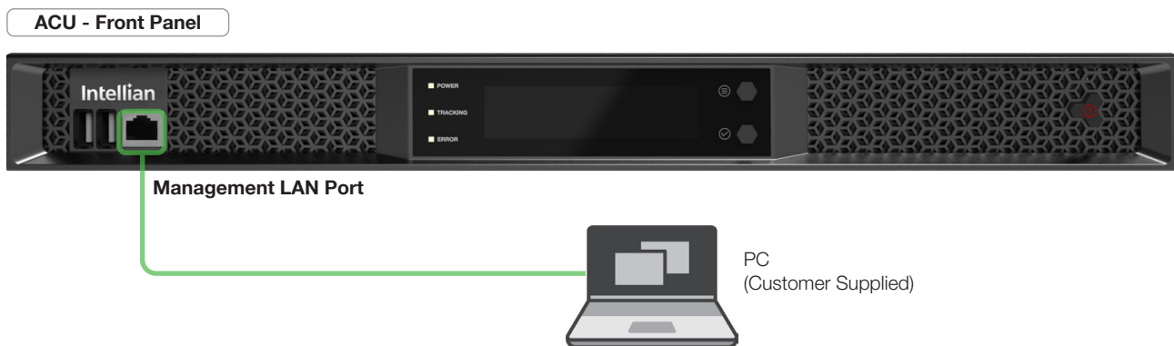
Figure 76: Front Panel Management LAN Port Connection
