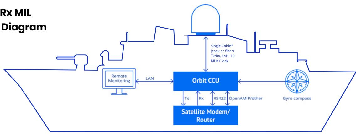
\*In case of simultaneous operation over more than one band, additional ADE-BDE cable will be required per band
