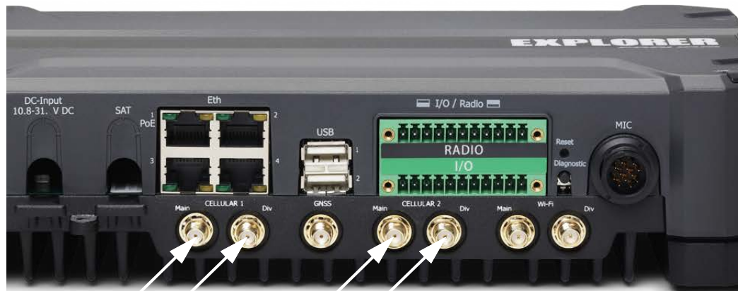
Figure 2-14: Connectors for cellular antennas
