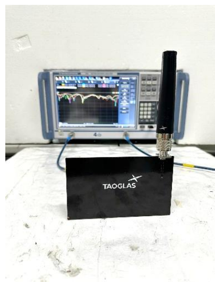
VNA Test Set-up – 15x9cm Ground Plane
