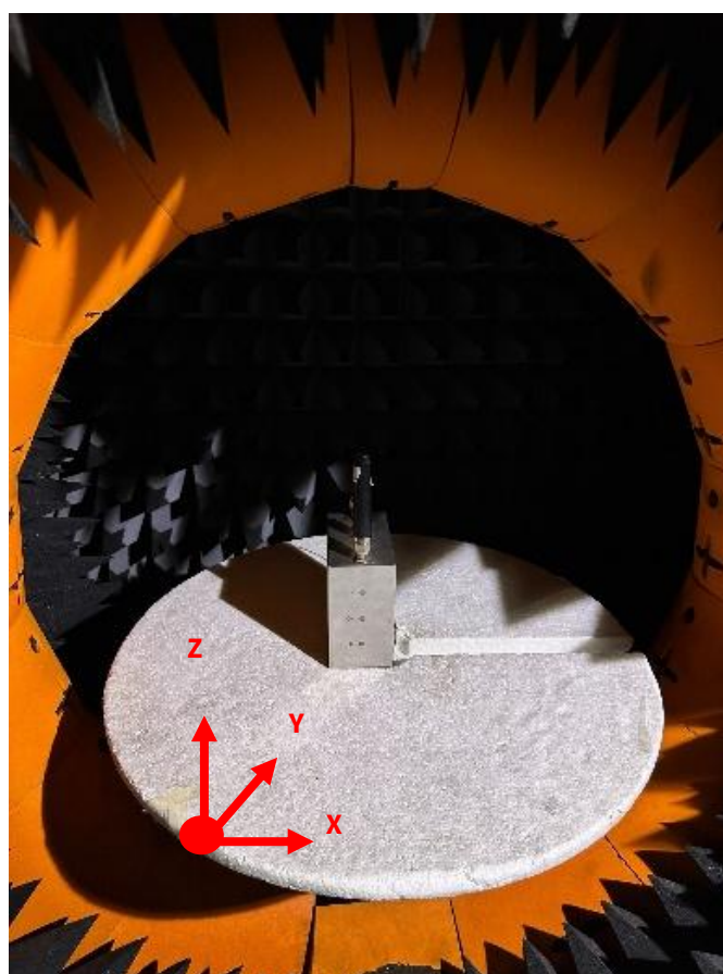
Test Set-up (The Metal box set up above represents a router set up)
