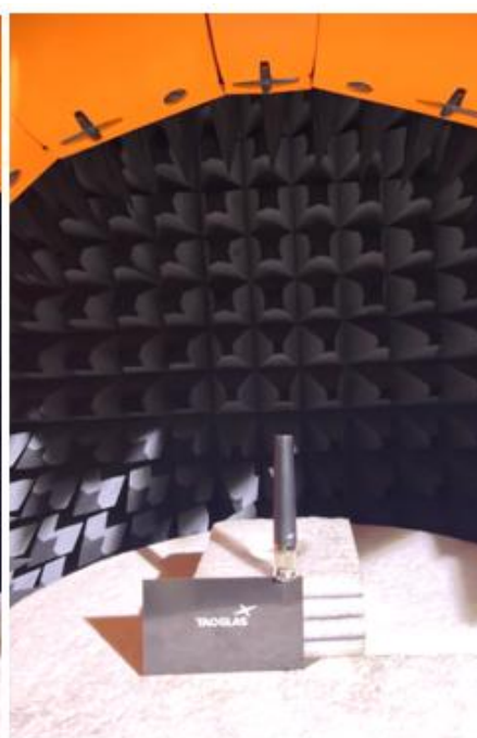
VNA Test Set-up – 15x9cm Ground Plane
