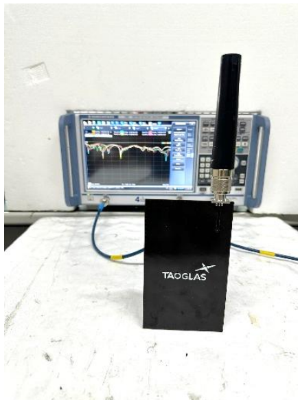
VNA Test Set-up – 9x15cm Ground Plane
