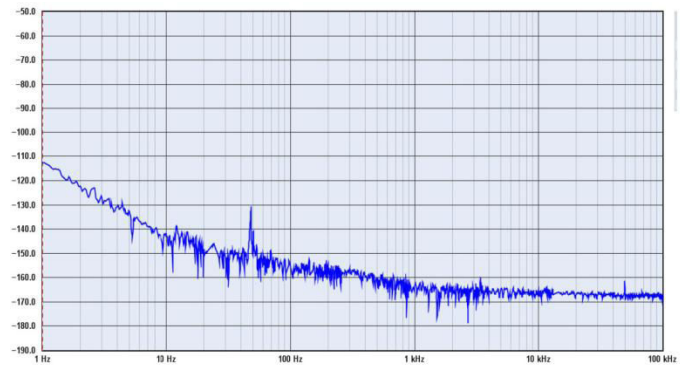
Typical MO ULN Phase Noise at 10MHz
