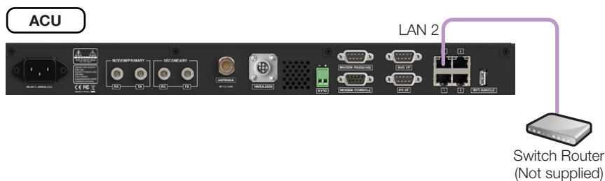
Figure 28: ACU to Switch Router Cable Connection
