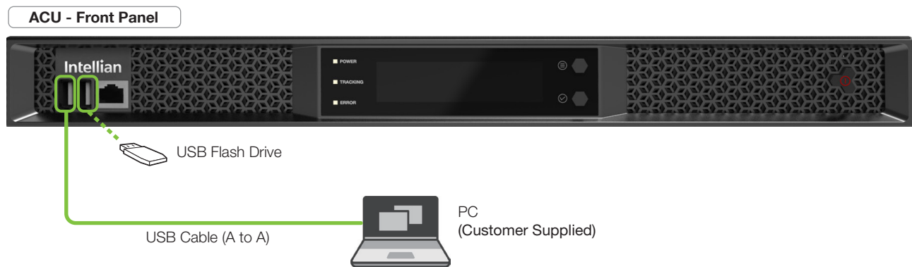
Figure 30: Front Panel USB Port Connection
