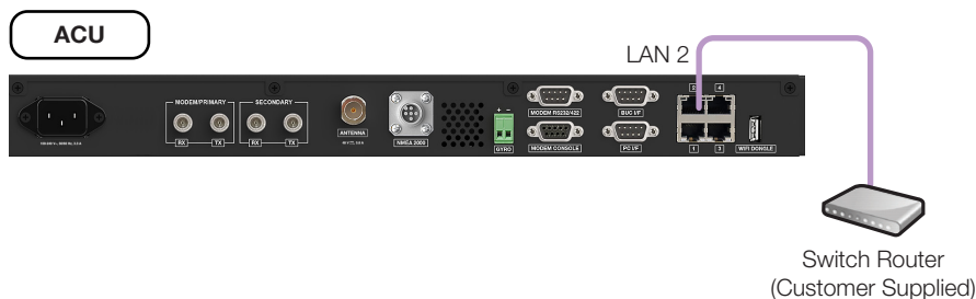
Figure 26: ACU to Switch Router Cable Connection
