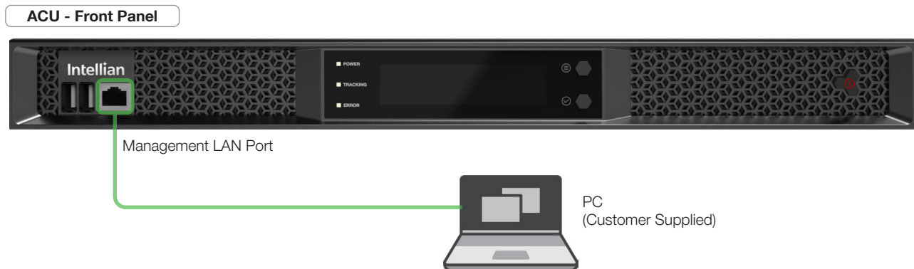
Figure 32: Front Panel Management LAN Port Connection
