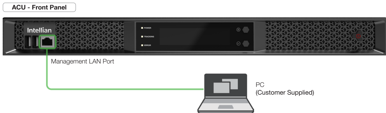
Figure 29: Front Panel Management LAN Port Connection
