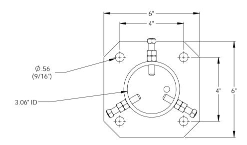
NOTE: ADAPTER TO SLEEVE OVER EXSITING 2.37"OD-3"OD MAST
