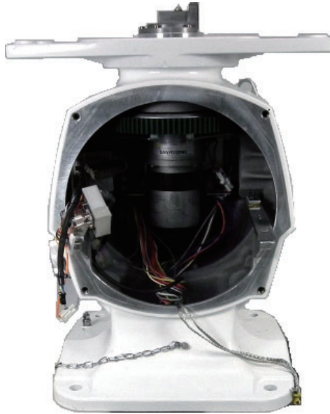
Rear view with cover and transceiver module RTR-101 removed.
