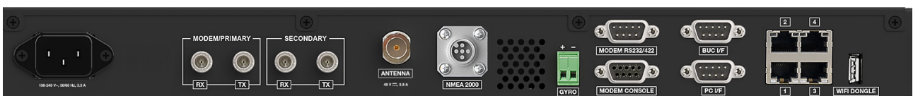
Figure 6: Back Panel of ACU
