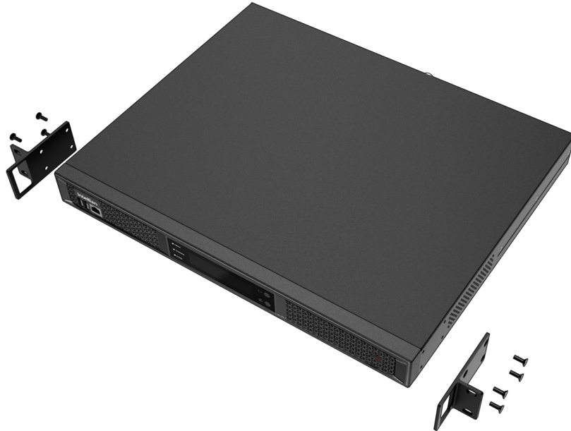
Figure 18: 19" Rack Mounting ACU
