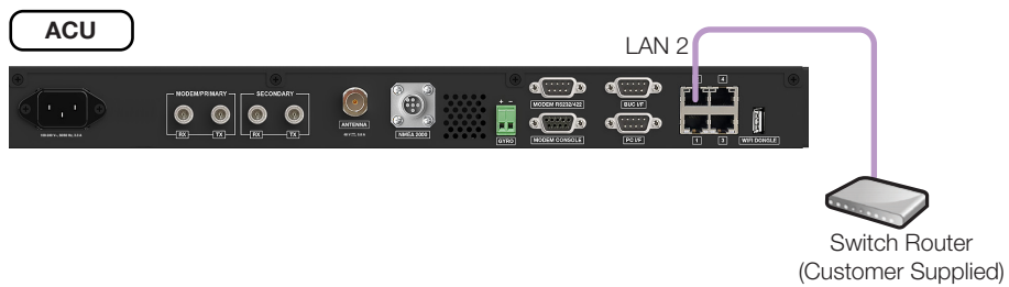
Figure 27: ACU to Switch Router Cable Connection
