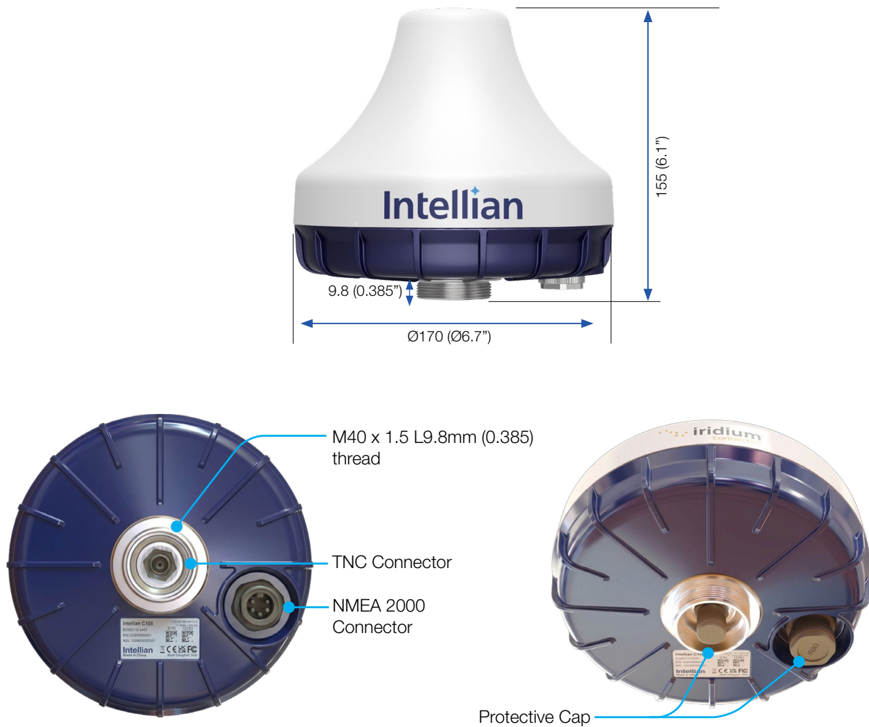
Figure 2: Antenna Dimensions
